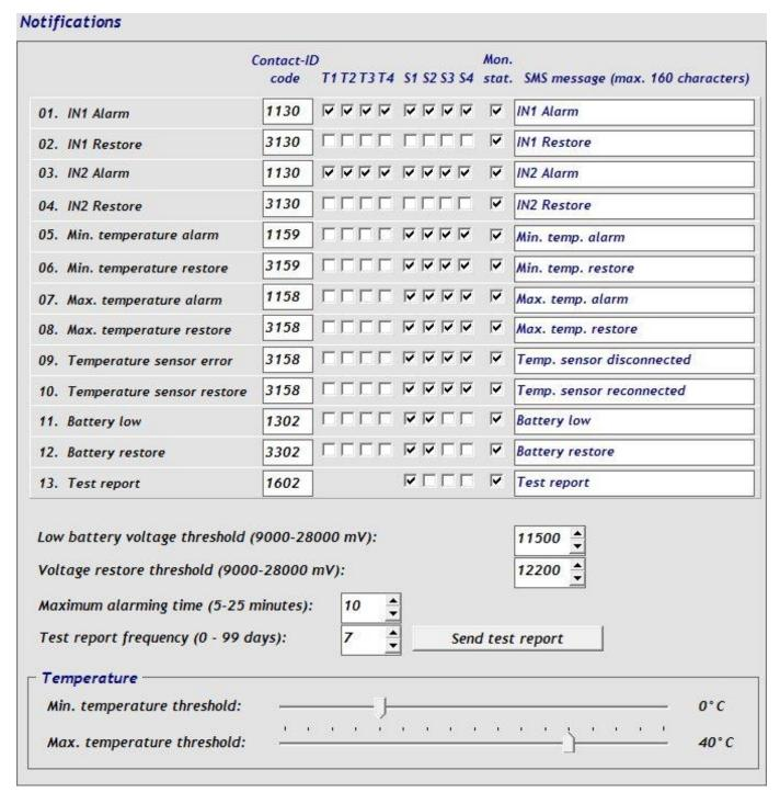
You can configure in the "Notifications" section which event to be reported to which user phone number by voice call (*T1-T4*) and/or SMS (*S1-S4*), and which event to be reported to monitoring station using Contact-ID protocol (*Mon. stat.*).
